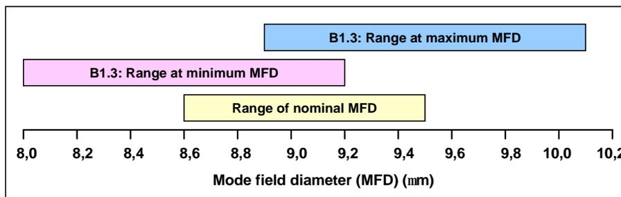
Figure 10 - Example spreads of mode field diameter (Type B1.3 SMF of [BS EN] IEC 60793-2-50:2008)
