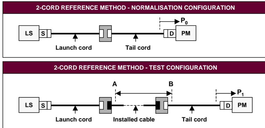
Figure A1 - 2-Cord Reference testing
