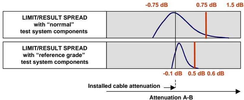
Figure A2 - Limits and spread of results using the 2-Cord Reference method (MMF)
