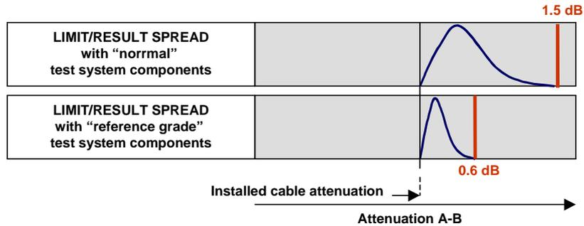
Figure 5 - Limits and spread of results using the 1-Cord Reference method (MMF)
