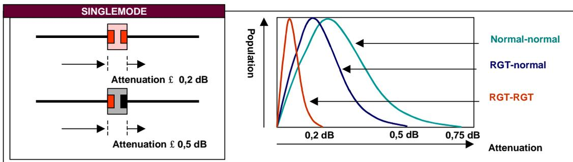
Figure 2 - Attenuation characteristic of singlemode terminations
