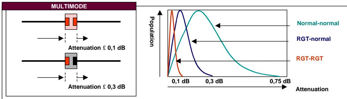
Figure 1 - Attenuation characteristic of multimode terminations
