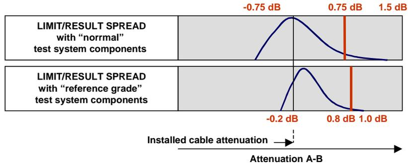
Figure A3 - Limits and spread of results using the 2-Cord Reference method (SMF)
