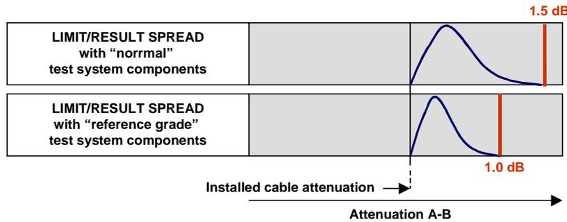
Figure 8 - Limits and spread of results using the 1-Cord Reference method (SMF)
