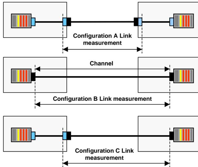
Figure 3 - Boundaries of measurement for channels and links
