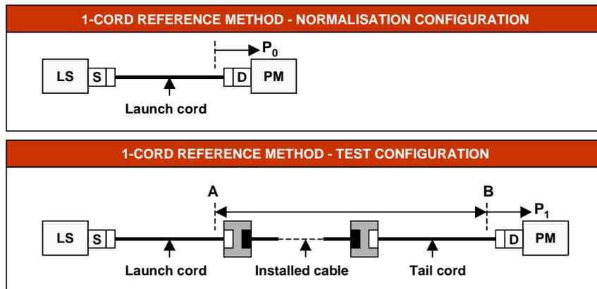
Figure 4 - 1-Cord Reference testing
