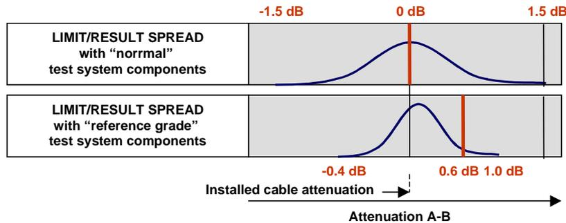
Figure 9 - Limits and spread of results using the 3-Cord Reference method (SMF)
