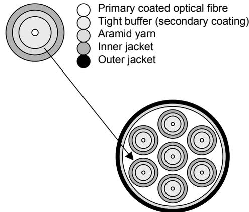
Figure 3: Breakout cables
