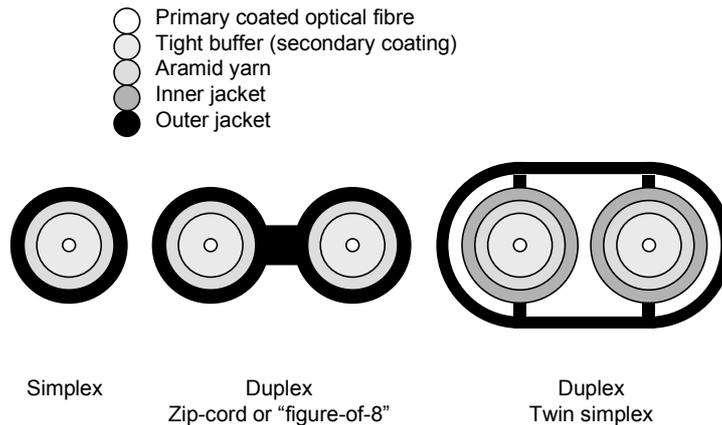
Figure 1: Patch and equipment cord cables
