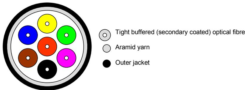
Figure 2: Internal distribution cables
