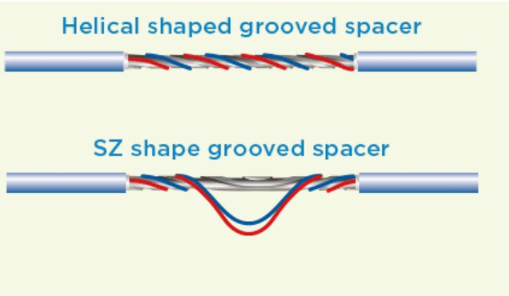
Mid-span breakout: helical versus SZ stranding design
